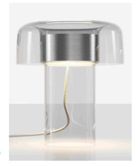
Tech. description The light comprises a glass shade surrounding a metal cylinder with a 24V LED module fitted on each side and a power cable with dimmer box, which houses the power source (LED driver), dimmer, and power switch. The dimmer allows adjustment of the brightness of the LED module and the direction of the light (up only, up and down, down only).
